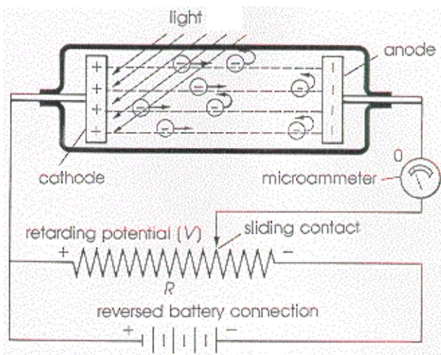
With the voltage set up in the opposite direction, Millikan could make the other electrode so negative that it would repel the photoelectron and prevent its movement across the tube. He called the necessary voltage the **cut off or stop voltage**. Thus, the electric potential established would have the same energy as the escaping photoelectron.
