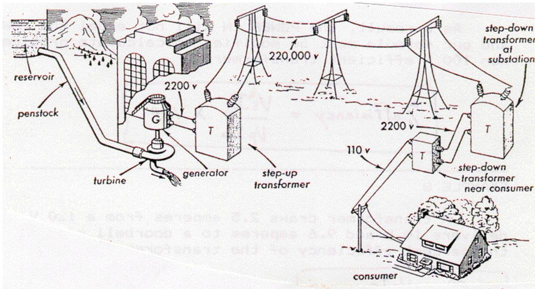
In the diagram above, at the generating station, electrical energy is passed through a step up transformer so that it can be transported over great distances through high voltage transmission lines. At a sub-station within a population center, the energy is passed through a step down transformer and transported over short distances down back alleys and underground to factories or homes. Every so often in the grid, the voltage is stepped down again to values that can be used in households.
