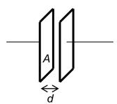
If a voltage is applied to a capacitor, say by connecting the capacitor to a battery, it quickly, although not instantaneously, becomes charged. One plate acquires a negative charge and the other an equal amount of positive charge. The amount of charge acquired by each plate is found to be proportional to the potential difference:
