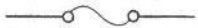
fuse (A fuse is a device that melts when the current in a circuit goes above a designed level. The melting fuse breaks the circuit.)
