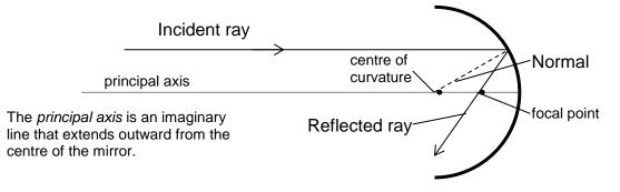
For a converging mirror, incident light rays which are parallel to the principal axis are reflected toward a <u>real</u> focal point.
