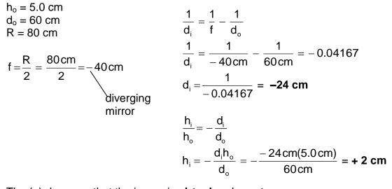
The (-) d<sub>i</sub> means that the image is **virtual** and **erect**. (All virtual images are erect.) The image is 2 cm tall, i.e. diminished.
