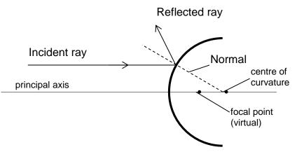
For a diverging mirror, incident light rays which are parallel to the principal axis are reflected away from a <u>virtual</u> focal point.
