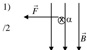
The Right Hand Rule (karate grip) is where fingers point in the direction of the magnetic field, thumb points in direction of the particle's initial motion, and the palm indicates the direction of the force.
