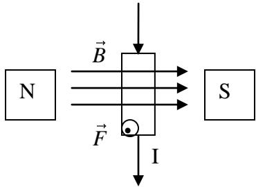
Using the Right Hand Rule, the fingers point in the direction of the magnetic field and the palm points in the direction of the force. The thumb indicates that the **current is flowing down the page.**
