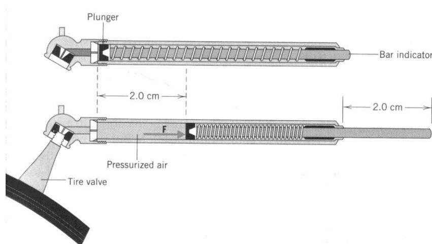
The force ( $F_s$ ) required to stretch or compress a spring is directly related to the stiffness of the spring (represented by the spring constant  $k$ ) and the amount that the spring is stretched or compressed ( $x$ ). The force supplied by a spring, elastic band, bungee cord, etc. can be calculated using a simple relation called Hooke's law (named after the efforts of Robert Hooke (1635 - 1662)).
