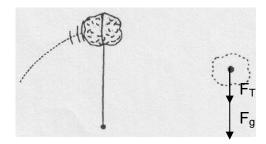
B. Tied to a post and moving in a circle at constant speed on a frictionless horizontal surface. Coming straight out of the paper.
